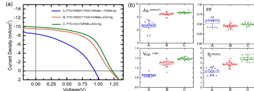
(a) Light current-voltage characteristics of PV devices with largest open-circuit potential ( $V_{OC}$ ) in all three device configurations under 1-sun illumination. (b) Box chart of device parameter distribution of all three device configurations: (A) FTO-PEDOT:PSS-FAPbBr<sub>3</sub>-PCBM-Ag, (B) FTO-PEDOT:PSS-FAPbBr<sub>3</sub>-ZnO-Ag, and (C) FTO-NiO-FAPbBr<sub>3</sub>-ZnO-Ag.
