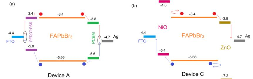
Energy band alignment diagram of planar FAPbBr<sub>3</sub> device depicting (a) possible pathways of charge recombination in device A due to band mismatch of organic transport layers, (b) efficient blocking mechanism on using inorganic charge-transport layers due to better band alignment (device C).
