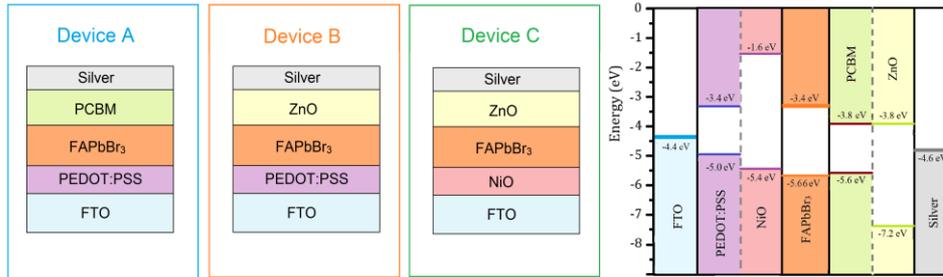
Device schematic of various configurations of planar p-i-n FAPbBr<sub>3</sub> devices using all-organic transport layers to all-inorganic transport layers. Energy band positions of different materials used in all three device configurations are also depicted.
