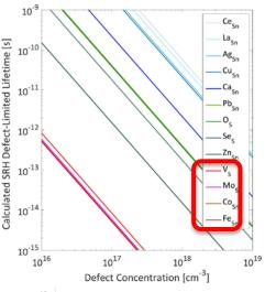
**Right:** Simulation (with WUStL) identifies four point defects (in red) as most detrimental to minority-carrier lifetime
