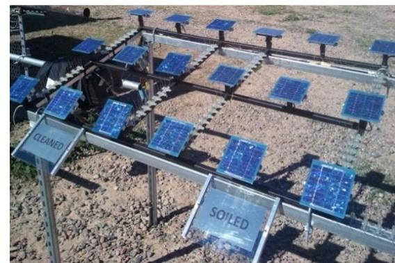
The apparatus that ASU and IITB developed for monitoring dust accumulation on test PV coupons as a function of tilt angle
