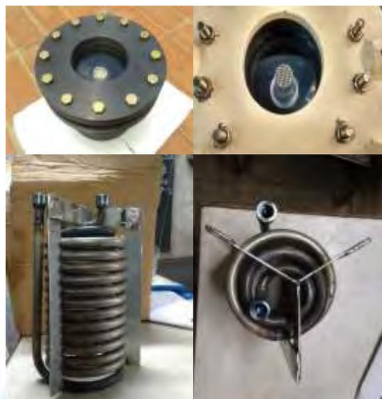
Figure 4: Small-scale helical coil receiver
