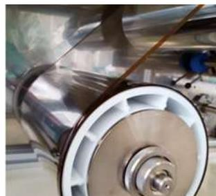
Corning® Willow® Glass flexible substrate – glass spool for roll-to-roll processing.
