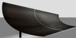
focused on supplying flexible glass substrates and technical support to enable the evaluation of disruptive PV material systems, device designs, and high-throughput fabrication methods. The flexible glass substrates are  $\leq 200\mu\text{m}$  thick and optimized for device substrate and hermetic barrier applications. The substrates are compatible with both sheet-based and roll-to-roll processes such as conveyance, vacuum deposition, solution coating, lamination, patterning, and printing.
