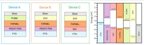
Device schematic of various configurations of planar p-i-n FAPbBr<sub>3</sub> devices using allorganic transport layers to all-inorganic transport layers. Energy band positions of different materials used in all three device configurations are also depicted.
