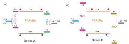
Energy band alignment diagram of planar FAPbBr<sub>3</sub> device depicting (a) possible pathways of charge recombination in device A due to band mismatch of organic transport layers, (b) efficient blocking mechanism on using inorganic charge-transport layers due to better band alignment (device C).
