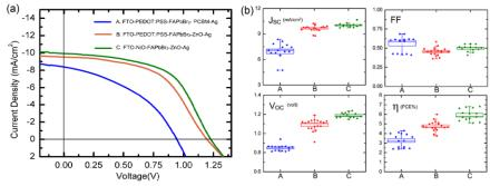
(a) Light current-voltage characteristics of PV devices with largest opencircuit potential ( $V_{OC}$ ) in all three device configurations under 1-sun illumination. (b) Box chart of device parameter distribution of all three device configurations: (A) FTO-PEDOT:PSS-FAPbBr<sub>3</sub>-PCBM-Ag, (B) FTO-PEDOT:PSS-FAPbBr<sub>3</sub>-ZnO-Ag, and (C) FTO-NiO-FAPbBr<sub>3</sub>-ZnO-Ag.
