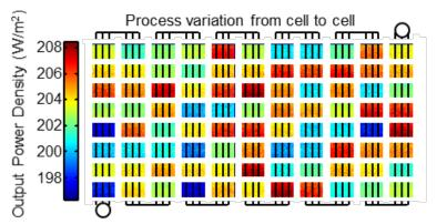
Output power density (W/m<sup>2</sup>) of a silicon HJ module. The cell-to-cell process variation can significantly impact the power that can be extracted from the module.
