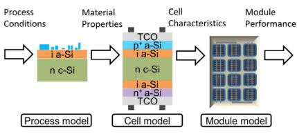
The end-to-end modeling framework for silicon heterojunction solar cell technology.
